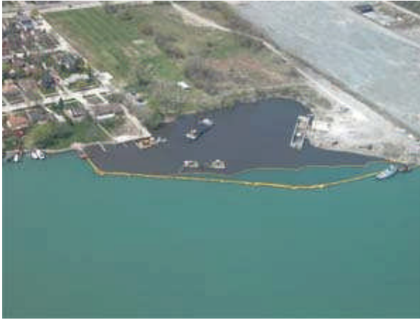
Figure 2. View of silt curtain surrounding Black Lagoon during remediation. Photo by Robert Burns, Detroit Riverkeeper.
